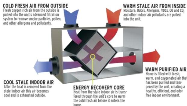
To maintain the ERV system, an access panel has been installed. Filters are to be cleaned every 3-6 months depending on living conditions (excess pet hair, dust etc.). **We recommend maintenance be done on the ERV unit by a mechanical professional on a quarterly basis.**
