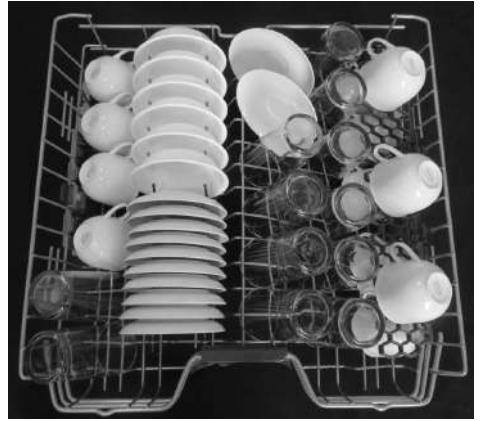
International Loading Pattern – Top rack (12 place settings)
