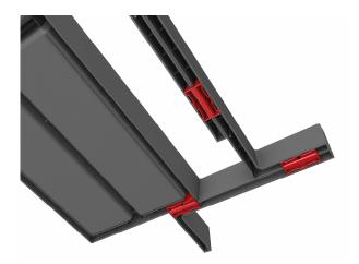
The connectors are installed by the underneath and hold 2 pieces together. They are then invsible once the set up is inserted in the drawer.
