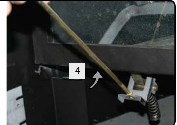
Figure 20.g Lift the door up and out of the fireplace frame
