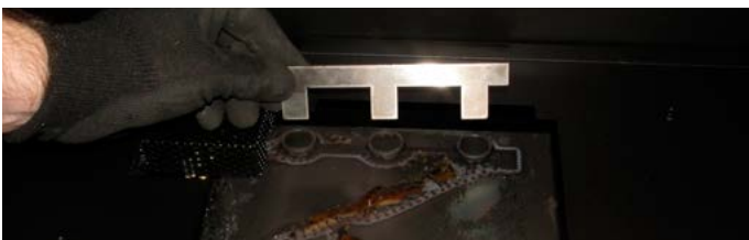
Figure 23.c Pushing the Rock Guard down into place.
